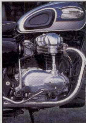
Unlike the new Triumph Bonneville, the Kawasaki W650 comes with a tachometer (above), kickstarter and knee pads (left). Camshaft is driven by a bevel-gear tower.
