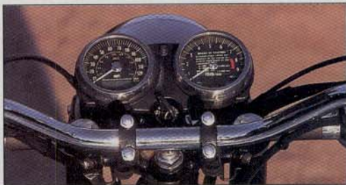
Unlike the new Triumph Bonneville, the Kawasaki W650 comes with a tachometer (above), kickstarter and knee pads (left). Camshaft is driven by a bevel-gear tower.
