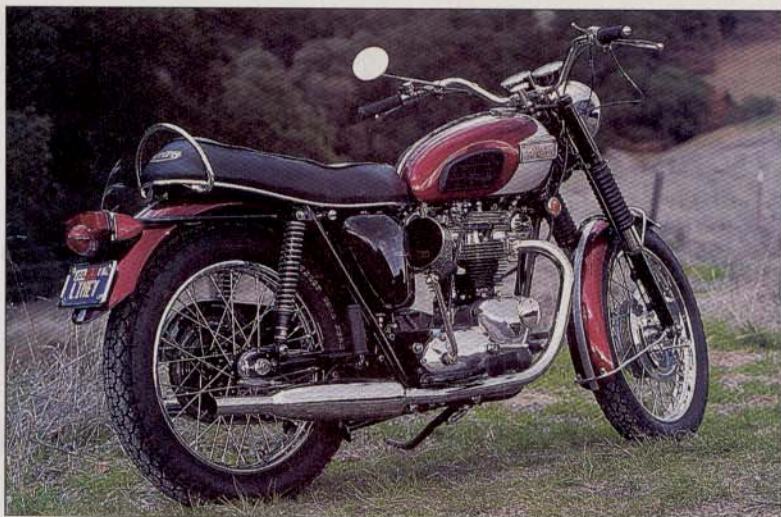
Standard equipment on the '69 Bonnie included (above) a pair of Smith's clocks, an ammeter and adjustable steering damper. Right: Later models had a unit engine and tranny.
