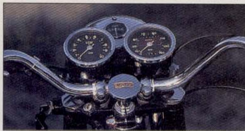
Standard equipment on the '69 Bonnie included (above) a pair of Smith's clocks, an ammeter and adjustable steering damper. Right: Later models had a unit engine and tranny.
