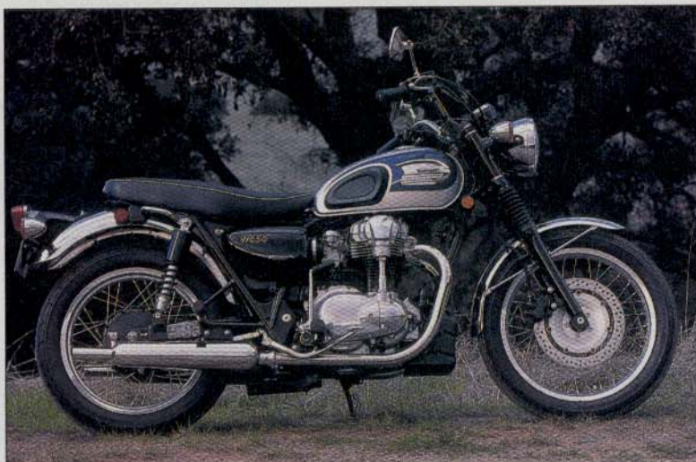
Unlike the new Triumph Bonneville, the Kawasaki W650 comes with a tachometer (above), kickstarter and knee pads (left). Camshaft is driven by a bevel-gear tower.
